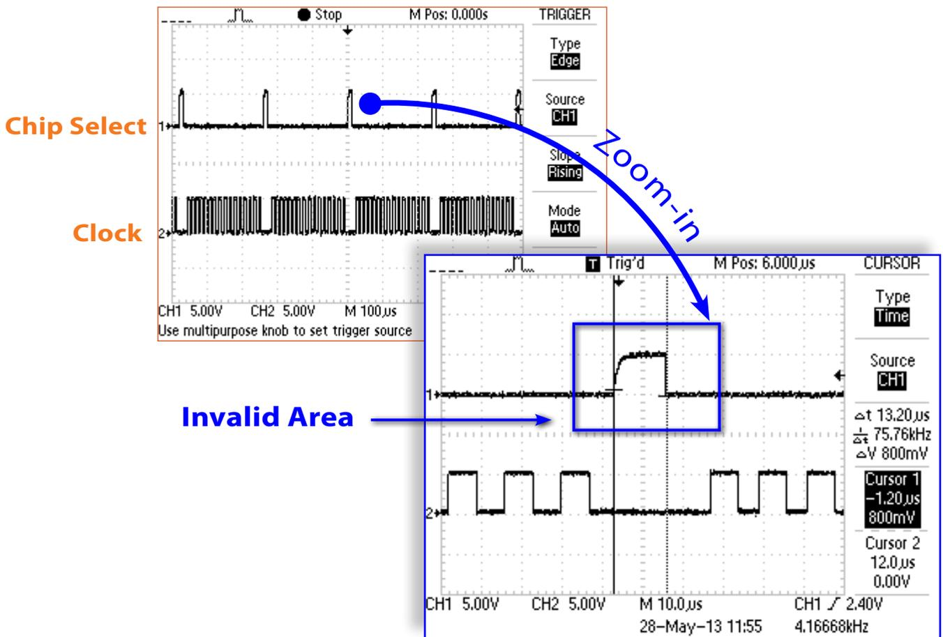
▲ Figure 3: SPI bus signal active low
