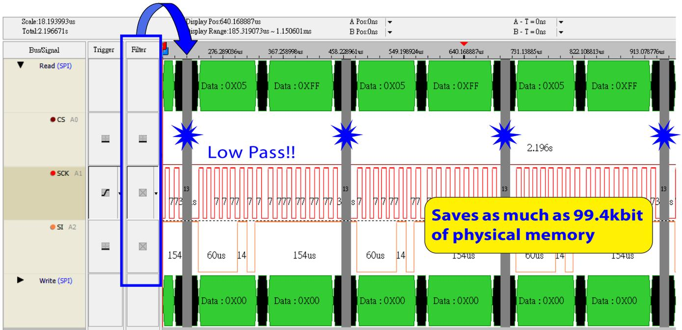
▲ Figure 4: The filter function of the logic analyzer can easily filter out unnecessary data
