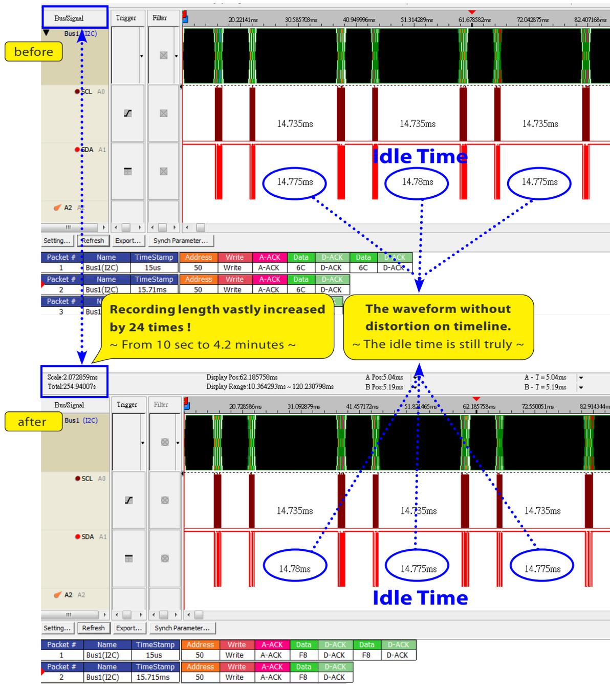
▲ Figure 2: Actual comparative testing of the ZEROPLUS Logic Analyzer (before and after compression)
