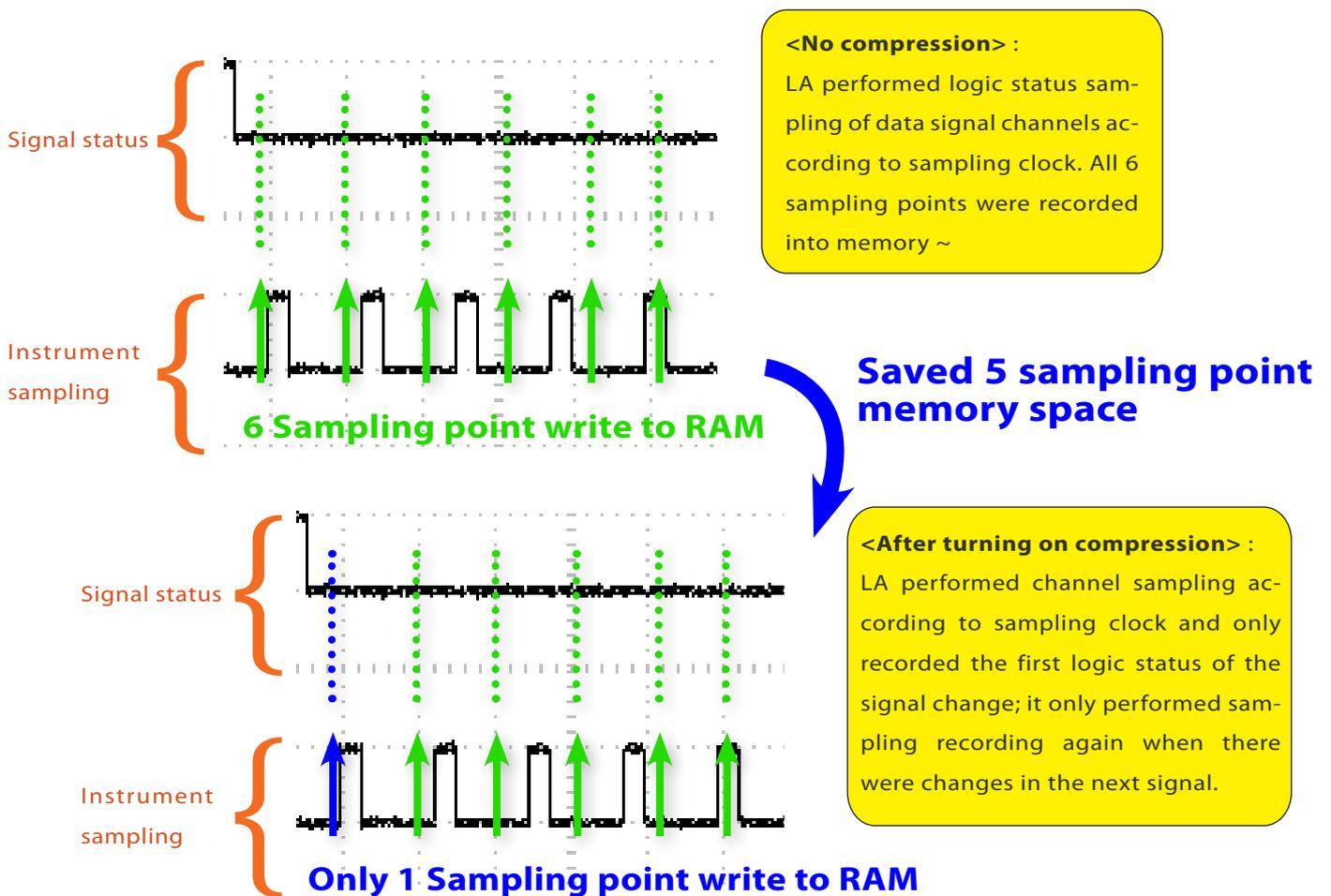
▲ Figure 1: Edge storage difference before and after turning on compression function.
