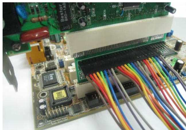
Figure 3: Use the PCI Measurement Fixture and the Test Cable of ZEROPLUS Technology
