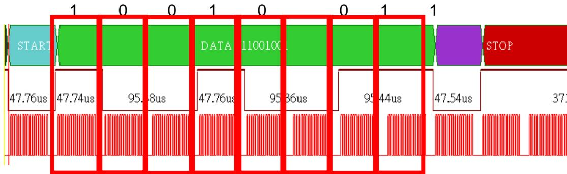
Figure 6: The Whole ISO7816 Signal Packet
