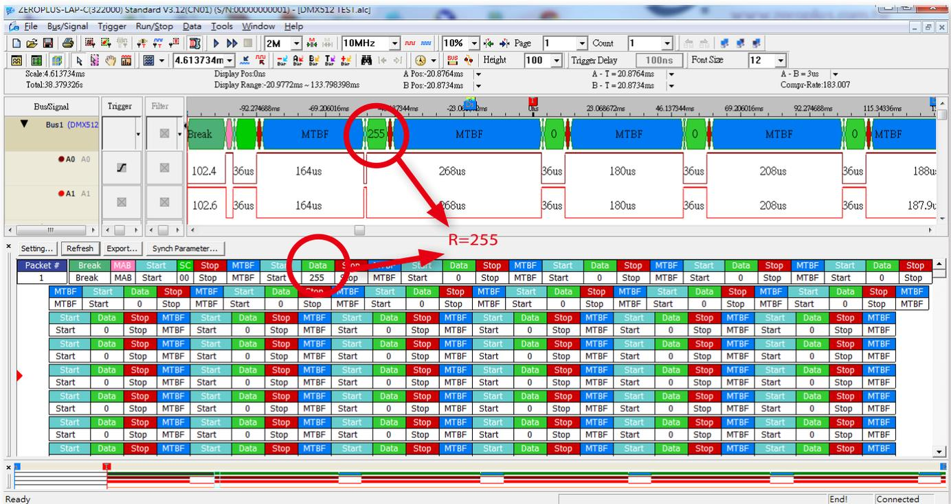
▲ Fig.4: DMX512 decoding of logic analyzer
