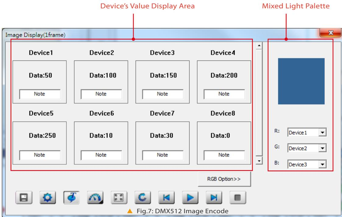
In the device's value display area, users can lock the device program to be analyzed and tracked and input the note of what the device is in the Note box. After the light sources of R, G, B and L have been set, the right mixed light palette can show the values of light sources and their mixed color. In this way, it is faster and more convenient for users to analyze the DMX512 network devices.
