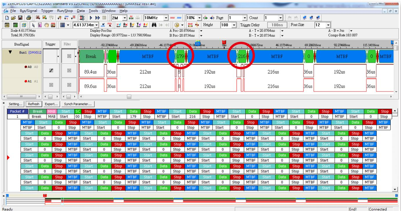
▲ Fig.6: DMX512 decoding of logic analyzer-R mixes with G.
