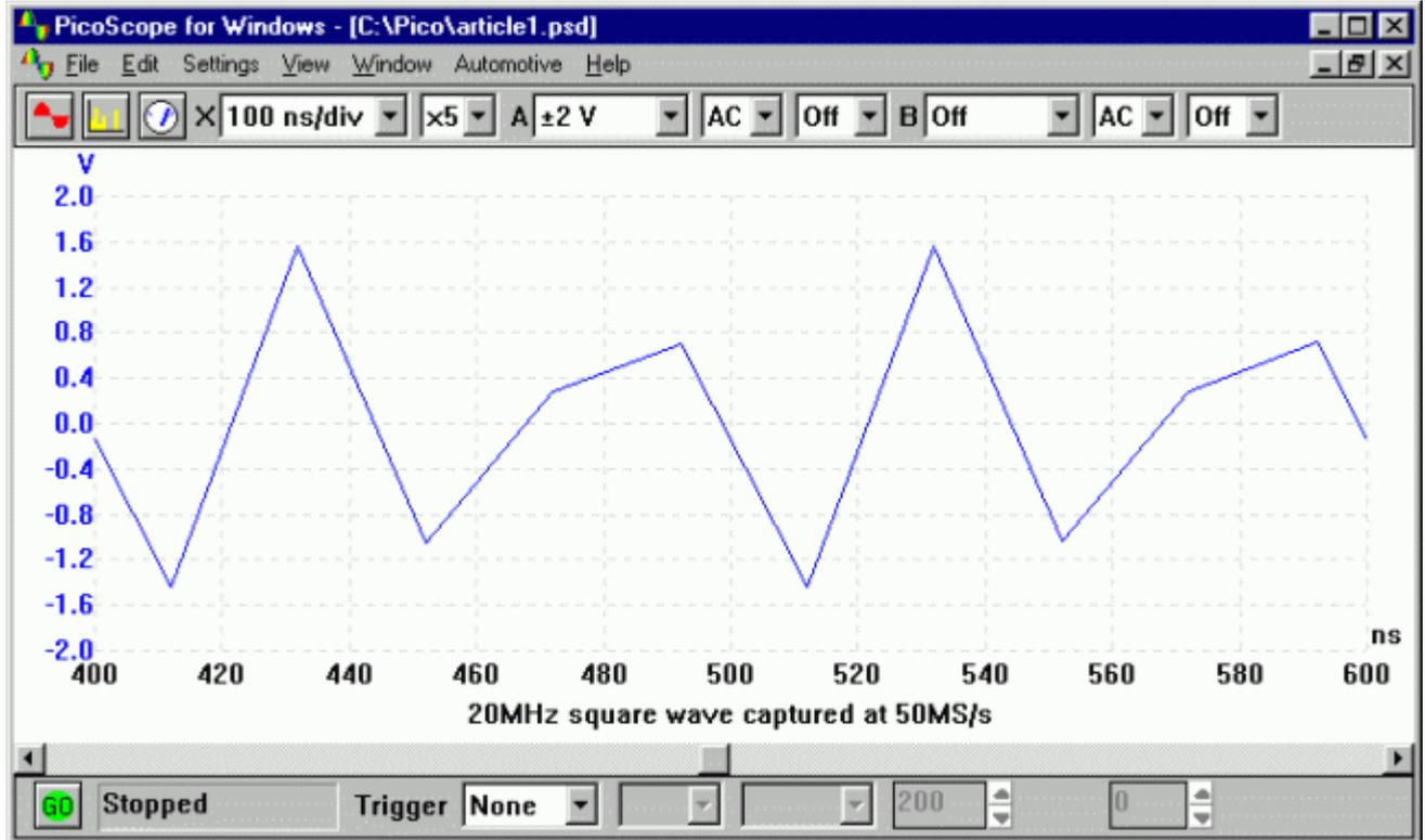
**Figure 1a: 20 MHz square wave captured with a sampling rate of 50 MS/s.**
