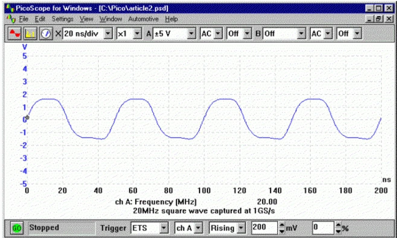
Figure 1b: 20MHz square wave captured at 1GS/s.
