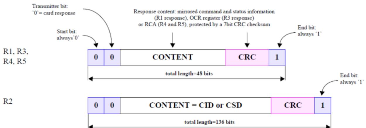
▲ **Fig.4: The basic response packet structure.**
