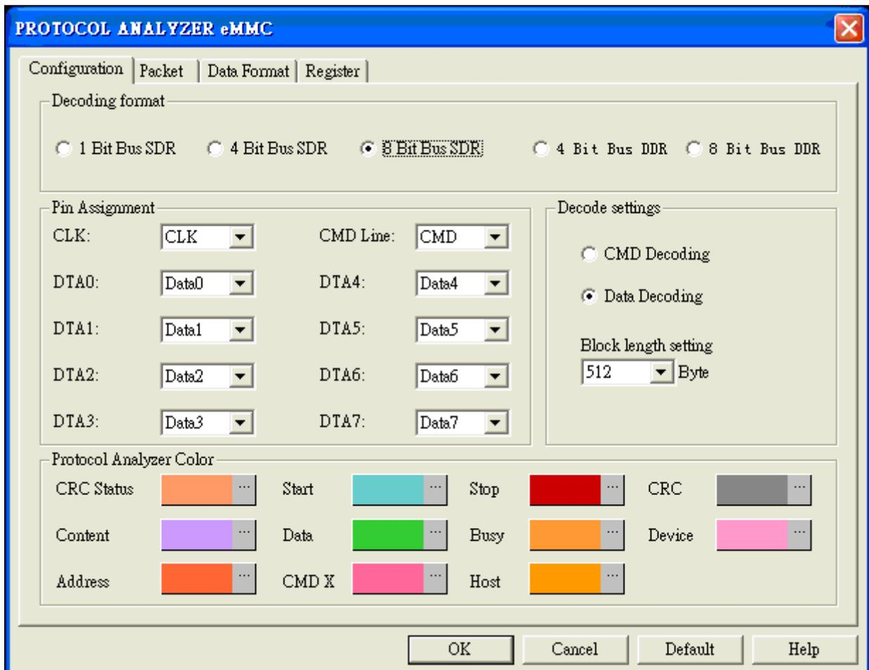
▲ Fig.9: eMMC Protocol Analyzer module setting window.
