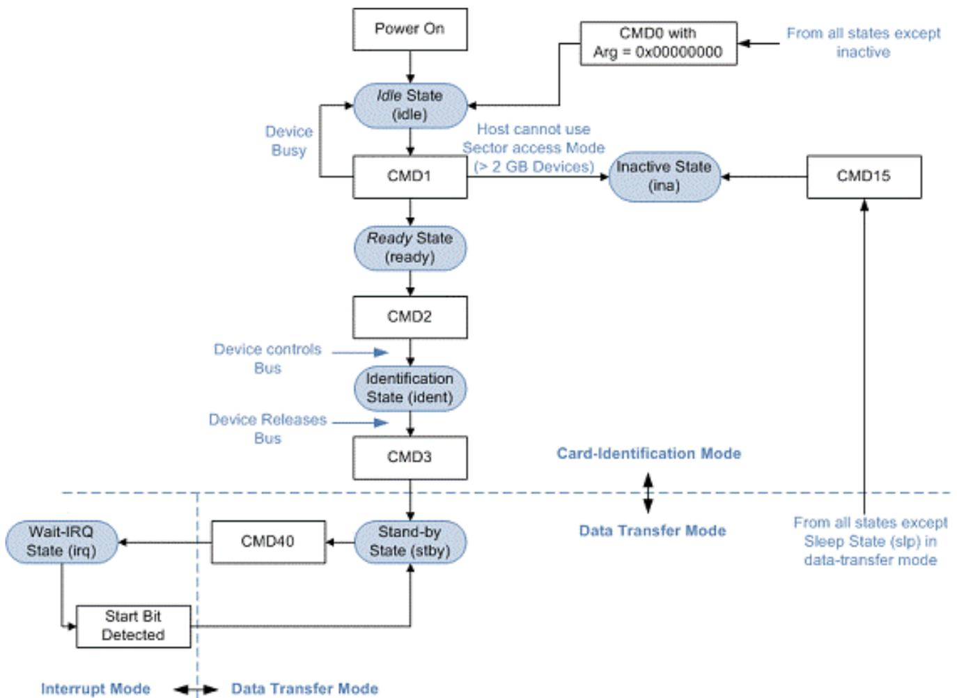
▲ Fig.3: State flow of eMMC card after power on (Identification Mode).
