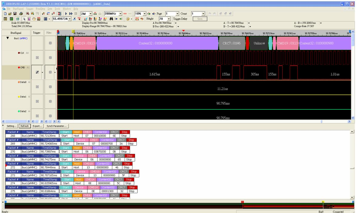
▲ Fig.7: Use Zeroplus Logic Analyzer to measure the eMMC CMD.
