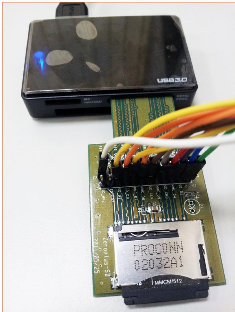
▲ **Fig.5: Connect the card reader and eMMC with the test line, then start the LA to capture.**
