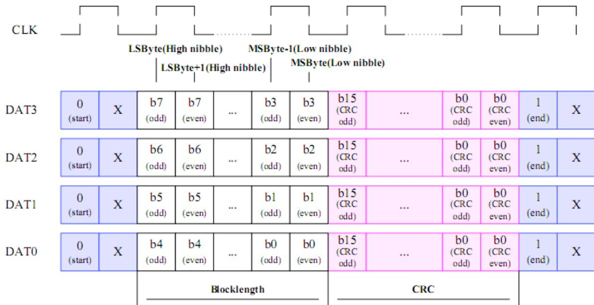
See below image for the DDR sampling mode. It captures the data at the rising/falling edge of CLK, to achieve double-data transmission. Please note that only the start bit and end bit are captured at the rising edge, the Data and CRC are captured at the rising/falling edge.
